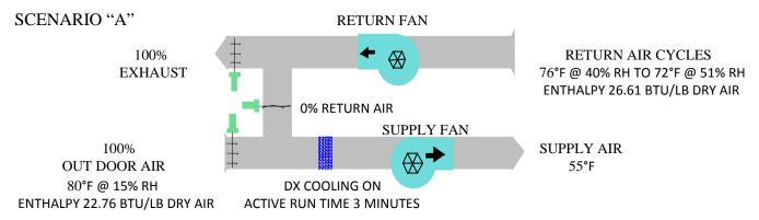
Scenario "A" illustrates a fan system, when the DX cooling compressor is active. Enthalpy comparison determines the heat content of the return air and outdoor air. The system dampers are on full outdoor air, as the total heat content of the outdoor air is approximately 14.5% less than the total heat content of the return air. Selecting the air stream with the lesser heat content causes the refrigeration compressor run time to be minimized.
