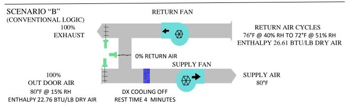
Scenario "B" illustrates the fan system, when the DX cooling compressor is not active. Enthalpy comparison determines the heat content of the return air and outdoor air. The dampers are on full fresh air, as the outdoor air contains 14.5% less total heat than the return air.
