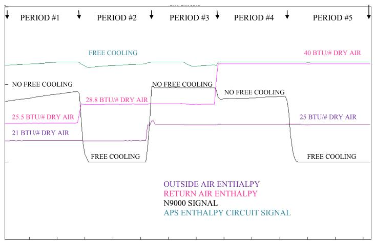
The above graph compares the performance of the Johnson Control N9000 Enthalpy Logic Module and the APS enthalpy comparison circuit.
