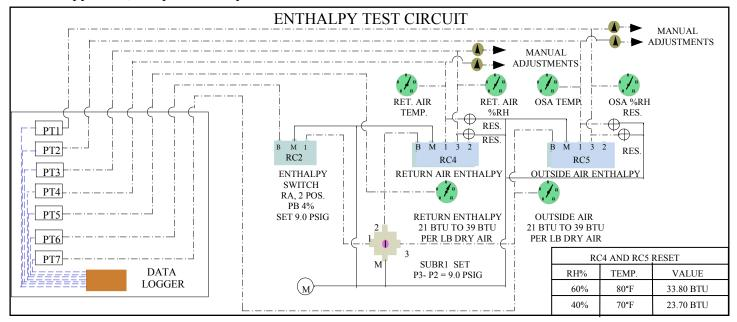
The Kreuter subtraction relay became obsolete; therefore, this circuit was developed allowing enthalpy comparison.
